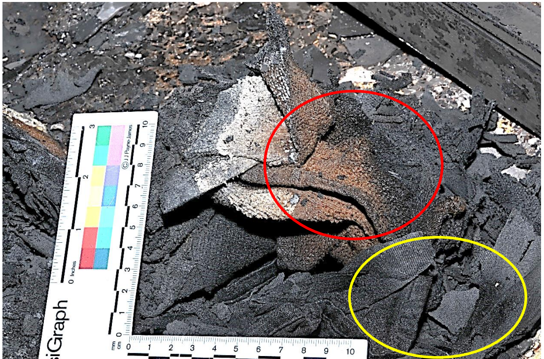
Image 1: The brown towelling material is visible in the centre of the image, (red ring). Also note the black, smooth cotton apron material to the bottom right of the image (Yellow ring) this has been converted to brittle carbon.
